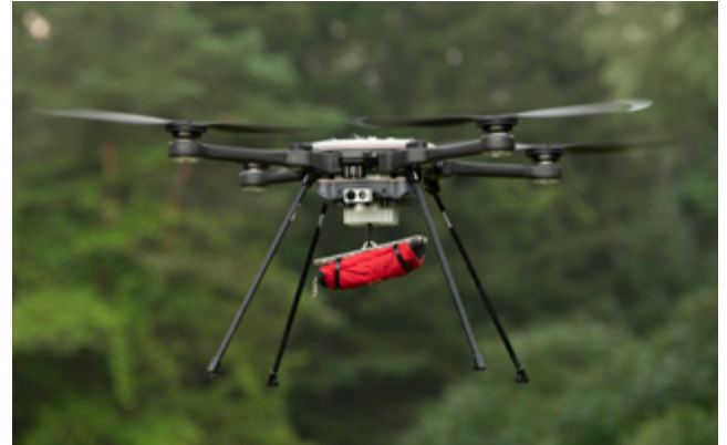
Easily attach, carry and deliver payloads up to 7.7 lbs
